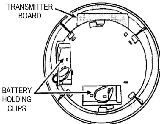
The smoke detector and transmitter are powered by two 9-volt alkaline batteries (supplied) which can power the unit for up to two years. If the battery voltage drops below normal, a low-battery report will be sent to the receiver with any status or alarm transmission. If a low-battery condition is indicated, replace *both* batteries. **NOTE:** Temperature and humidity extremes may reduce the life of the battery.
